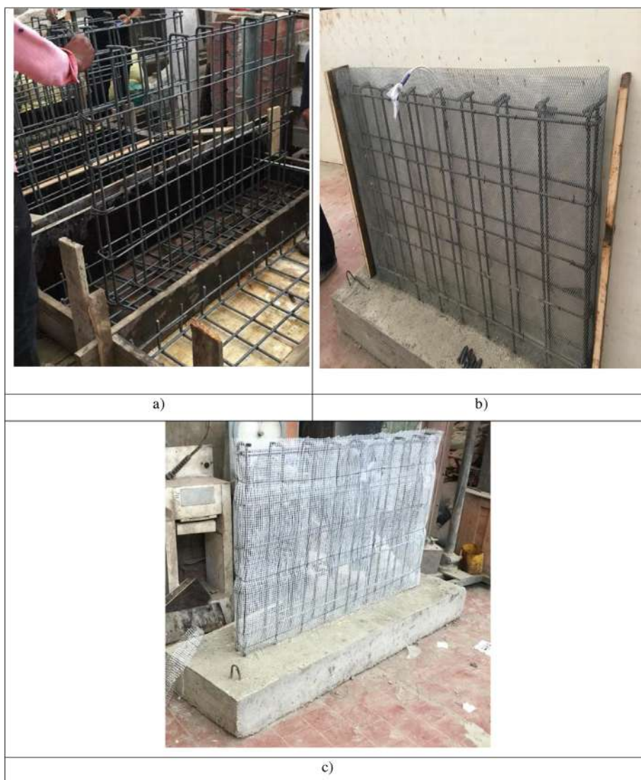
Fig. 4. Specimen configurations: (a) control wall; (b) wall with expanded wire mesh; (c) wall with glass fiber mesh.
